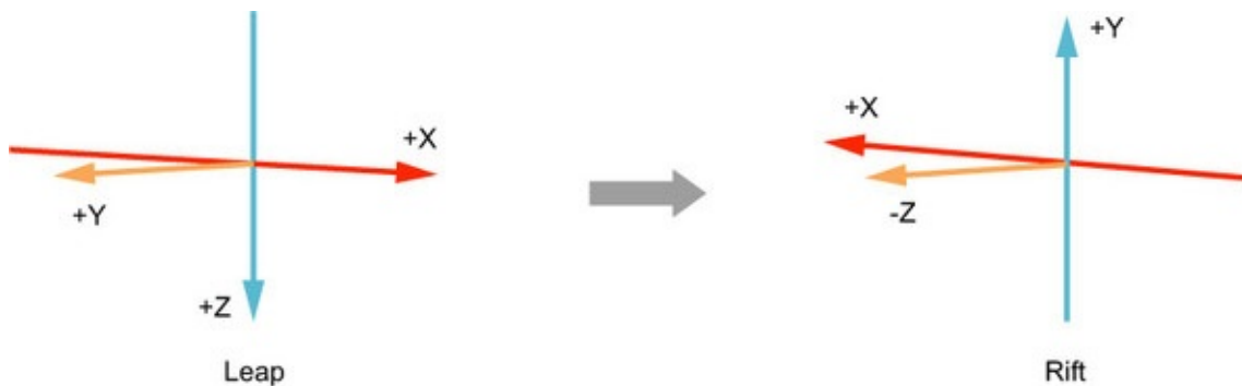
Figure 13.15. Transformation from Leap coordinates to Rift coordinates
