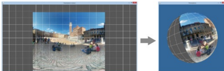
Figure 13.4. Wrapping a partial photo texture onto a sphere. The image used here is a photo sphere taken of the same plaza as the panorama shot in figure 13.1 .
