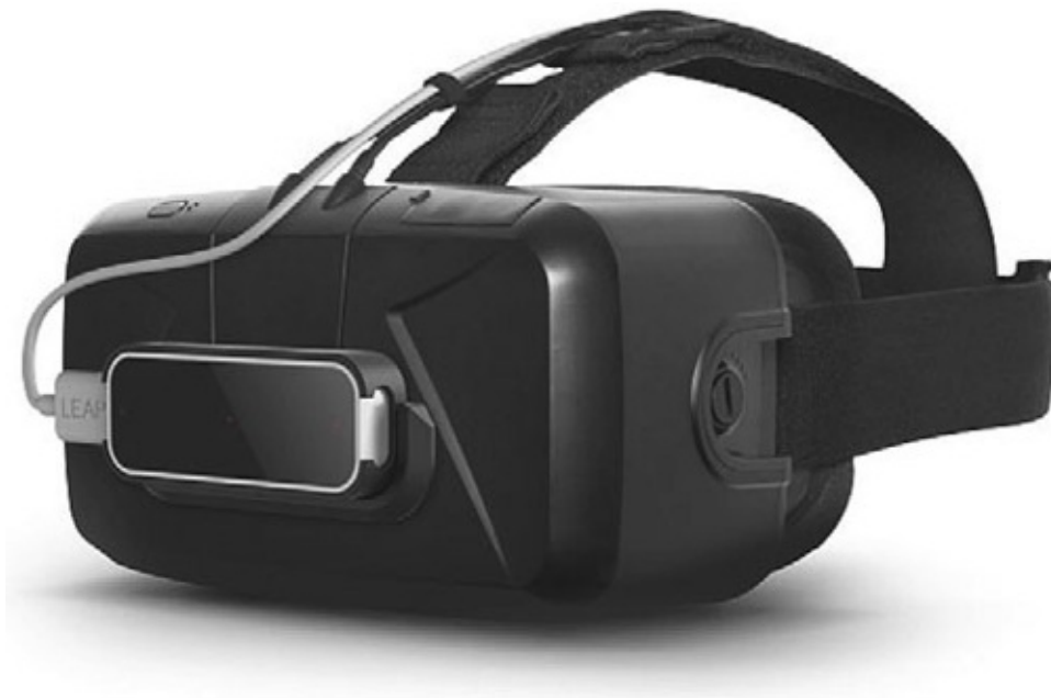
Figure 13.12. An Oculus Rift DK2 with the Leap Motion mounted on a removable bracket attached to the faceplate. The Leap can be popped out of the bracket holder and doesn't block the Rift's IR LEDs.
