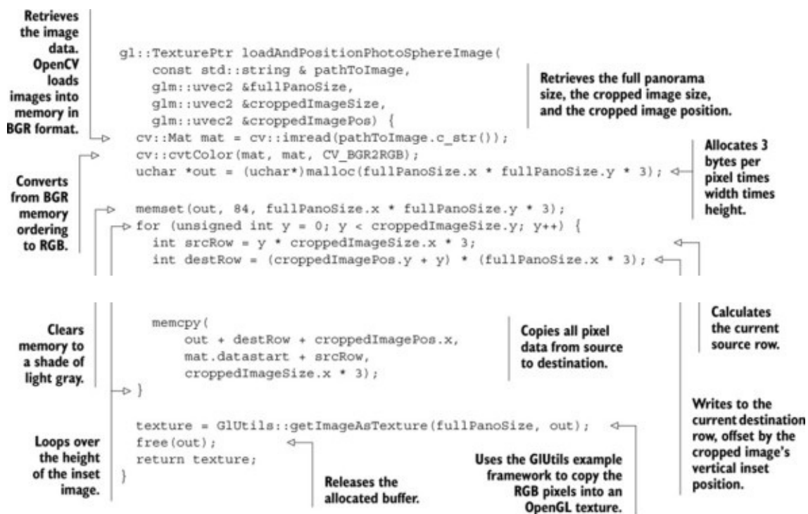
Listing 13.2. Using OpenCV to load an image, and then embedding it into a texture
