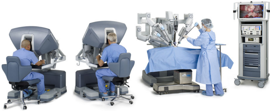
Fig. 4.45 Robotic surgery with the telemanipulation system “da Vinci”, © 2011 Intuitive Surgical, Inc. [38, 76]
