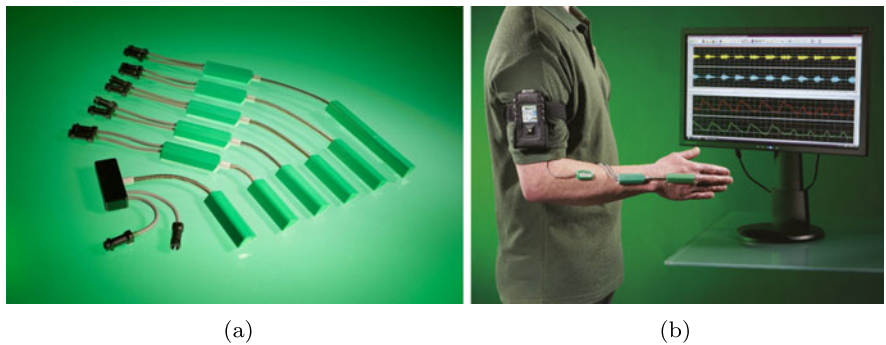
Fig. 2.3 Twin Axis Goniometers; by courtesy of Biometrics Ltd. ( www.biometricsltd.com )
