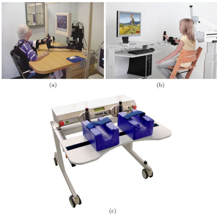
Fig. 7.4 Examples of arm rehabilitation robots. (a) MIT-Manus used for therapy at Burke Rehabilitation Hospital (White Plains, NY), originally published in [31]; with kind permission from Springer Science+Business Media B.V.; (b) Armeo@Spring Pediatric, Hocoma AG, Switzerland; (c) Bi-Manu-Track, by courtesy of B. Brandl-Hesse
