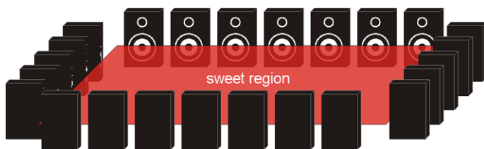
Fig. 5.5 In a wave field synthesis system the "sweet spot" location is extended to a "sweet region". Within this region the listener gets the impression of being within a genuine sound field indistinguishable from a real sound field
