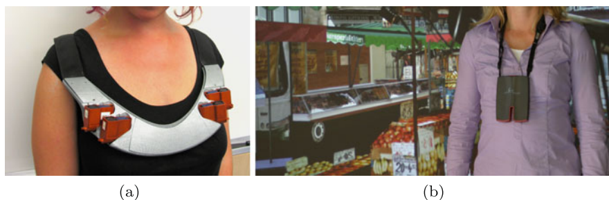
Fig. 6.3 Wearable olfactory displays. (a) ICT Scent Collar, by courtesy of J. Morie, University of Southern California; (b) Sniffman in combination with virtual marketplace; by courtesy of S. Beckhaus, University of Hamburg
