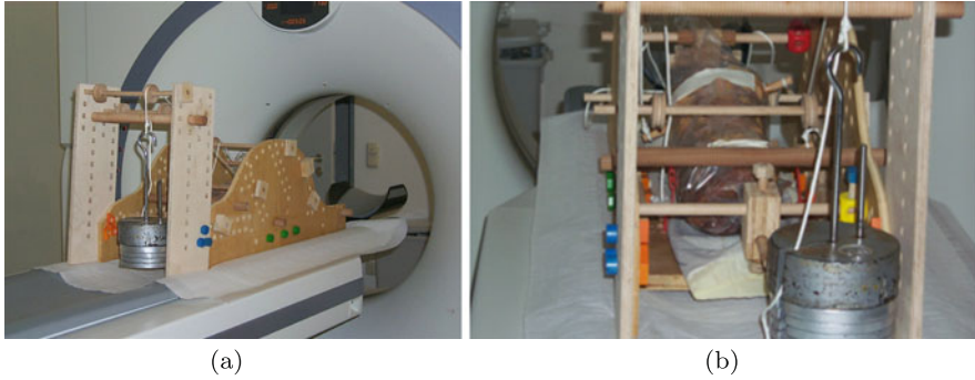
Fig. 8.13 Image data acquisition; by courtesy of Rainer Burgkart, TU München. (a) Setup for CT recordings; (b) The wooden construction enables the adjustment of different knee postures
