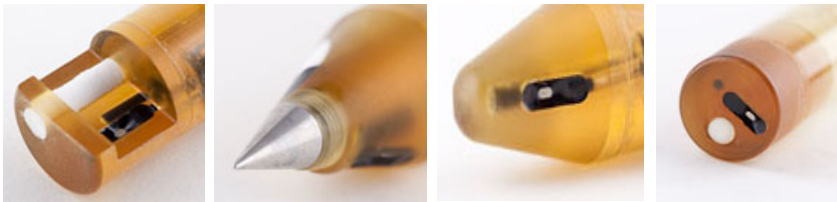
Fig. 7. Location the ISFET sensor in the pH electrode [10]
